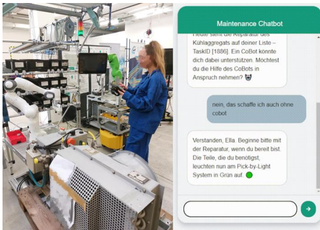
Figure 5: Maintenance of a railway cooling system using a chatbot
