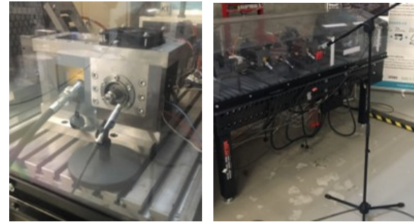
(a) Microphone inside the safety cover, referred to as IntMic . (b) Microphone outside the safety cover, referred to as ExtMic .
