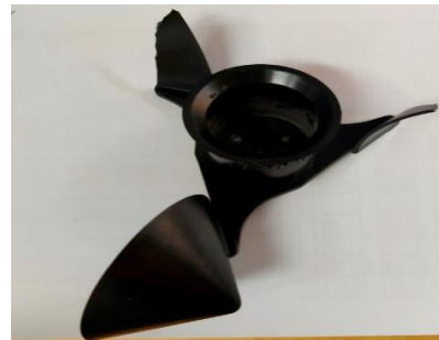
Fig. 1 Breakage of the Anemometer cup
