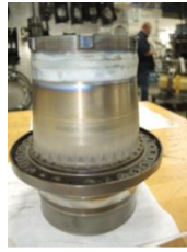
Figure 4. Expensive secondary damage to stub shaft
