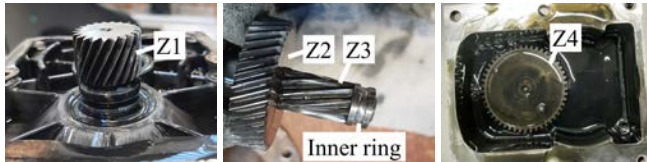
Figure 5. Failure of gearbox H45. Shown are the gears from left to right Z1 and Z2 with minor wear, Z3 with moderate wear and Z4 along with the gearbox full of the deteriorated oil. As well as the destroyed bearings inner ring next to Z3.
