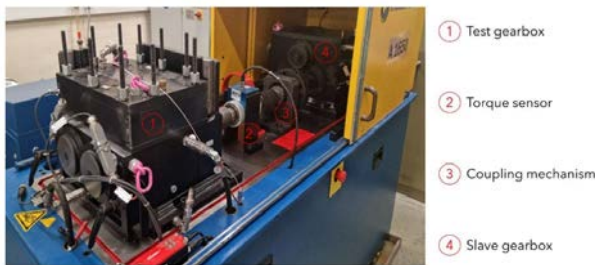
Figure 3. Photo of the multistage FZG test rig
