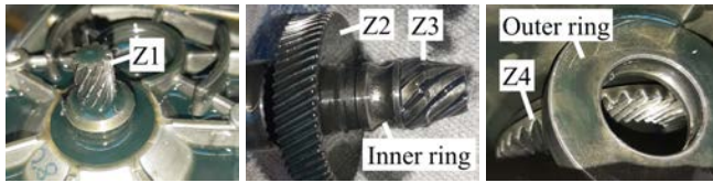
Figure 4. Failure of gearbox B45. Shown are the gears from left to right Z1 with moderate wear, Z2 with minor wear, Z3 with destructive wear and Z4 with moderate wear. As well as the destroyed bearings' inner ring next to Z3 and outer ring next to Z4.
